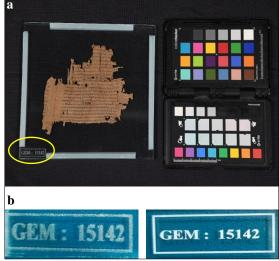
Figure (4) Shows **<u>a</u>**. numbering with CO<sub>2</sub> laser marker machine on glass mount; then putting the papyrus was between glass sheets, **<u>b</u>**. final results of numbering by CO<sub>2</sub> laser marker machine (*left*) and U.V laser printer (*right*).
