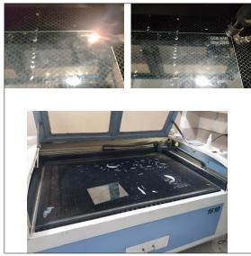
Figure (3) Shows numbering with  $CO_2$  laser marker machine, (the glass mount was numbered separately, by the authors.
